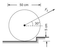
Compute the forces  $F_1$  and  $F_2$  required to just start a 100 kg lawn mower over a 5 cm step when
