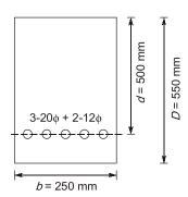
1.6 Determine limiting moment of resistance and maximum percentage of steel required for the concrete cross-section shown in figure below. Use limit state method, and M15 and Fe415 steel.
