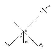
1.7 A smooth right circular cylinder of radius 0.5 m rests on a horizontal plane and is kept from rolling by an inclined string AC of length 1.0 m. A prismatic bar of length 1.5 m and weight 125 N is hinged at point A and leans against the cylinder as shown in the figure below. Find the tension S that will be induced in the string AC.
