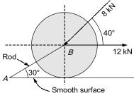
Let  $F_{AB}$  be the force in the rod AB and B be the reaction from floor.
