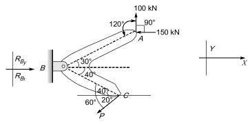
Let  $R_{Bx}$  and  $R_{By}$  be the reaction component at B in X and Y direction respectively.
